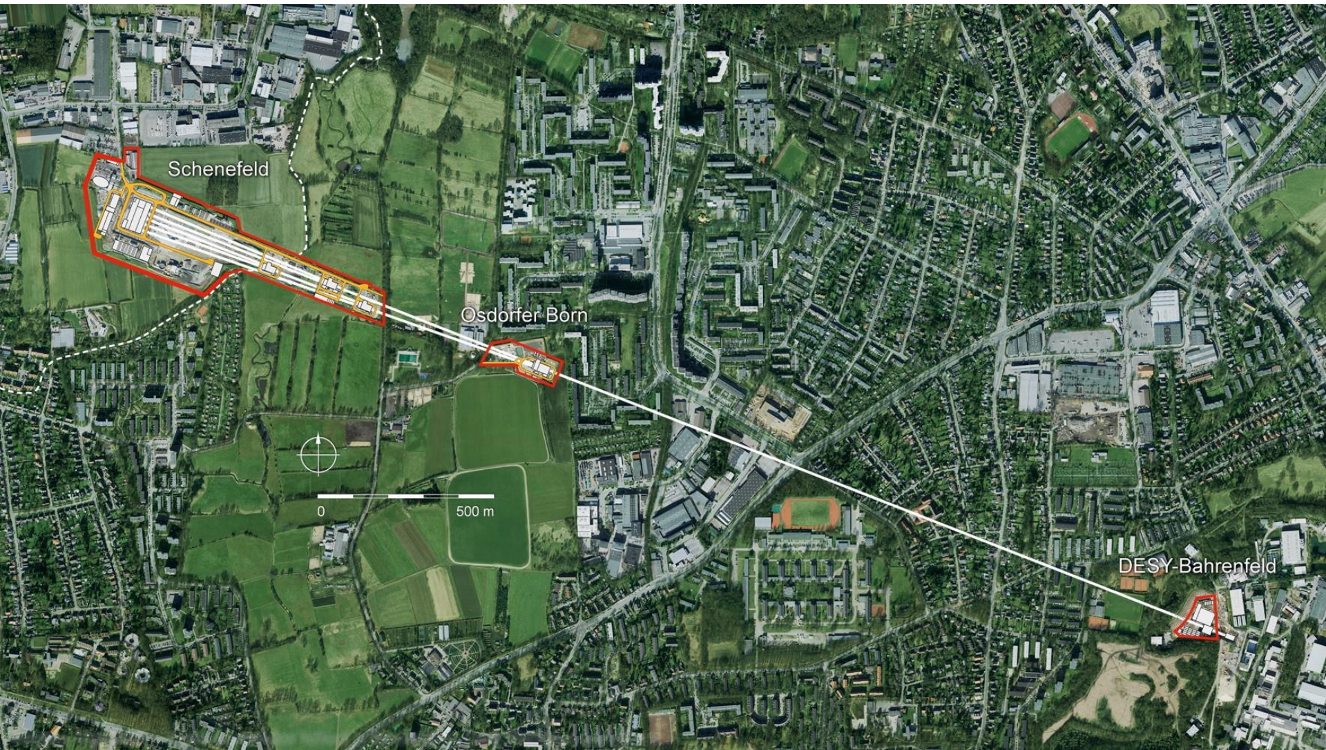
European superconducting E-XFEL at DESY, Hamburg: 3.4 km long, E = 17.5 \text{ GeV} , \tau = 5\text{-}85 \text{ fs}
