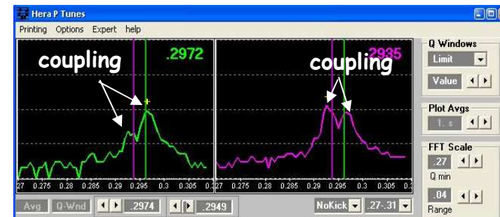
HERA p tune spectrum (repetitive chirp excitation & resonant „Schottky type“ pick-up)
