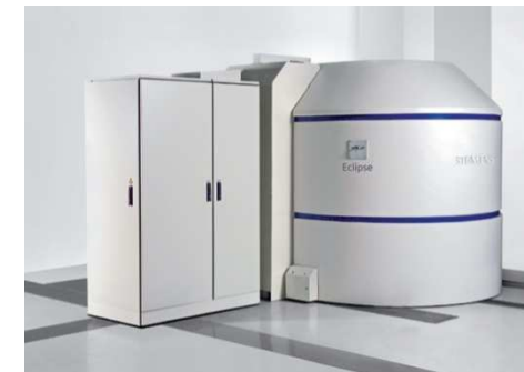
Siemens Eclipse Cyclotron (11 MeV) marketed for PET isotope production
