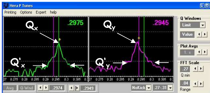
HERA p tune spectrum (repetitive chirp excitation & resonant „Schottky type“ pick-up)
