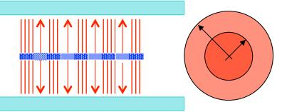
In the case of charge distribution, and  $\gamma \rightarrow \infty$ , the electric field lines are perpendicular to the direction of motion. The transverse fields intensity can be computed like in the static case, applying the Gauss and Ampere laws.
