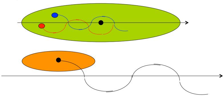
These force may have a complicate dependence on the charge position. A simple analysis is done considering only the linear expansion of the self-fields forces around the equilibrium trajectory.
