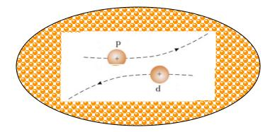
2) Space Charge Regime ==> dominated by the self field produced by the particle distribution, which varies appreciably only over large distances compare to the average separation of the particles ==> Collective Effects
