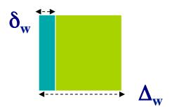
The skin depth depends on the material properties and on the frequency. Fields pass through the conductor wall if  $\delta_w > \Delta_w$ . This happens at relatively low frequencies.
