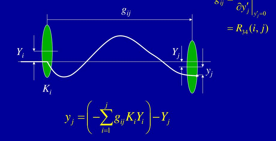
linear system: just superimpose oscillations caused by quad kicks.
