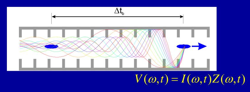
Bunch 'current' generates wake that decelerates trailing bunches.
