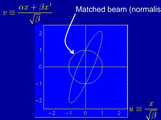
Mismatched beam ( $\beta$ -mismatch) rotates with nominal phase advance along beamline
