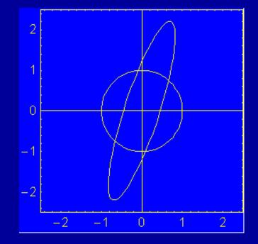
Mismatched beam (β-mismatch) rotates with nominal phase advance along beamline
