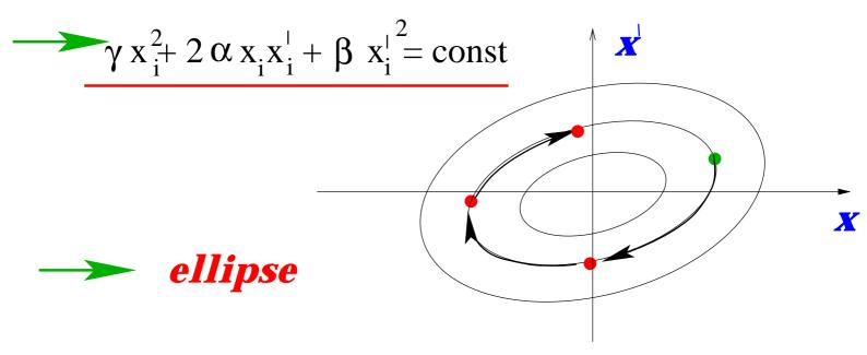
the ellipse orientation and the half axis length vary along the machine
