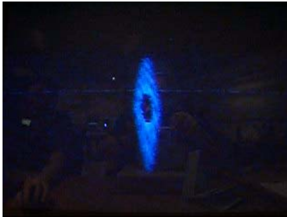
Synchrotron Radiation Profile Monitor (SRPM) showing the transverse beam shape
