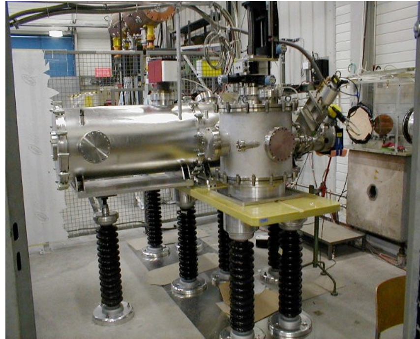
The prototype Laser Ion Source in building 236 on a HV platform (~100 kV) to decrease space charge
