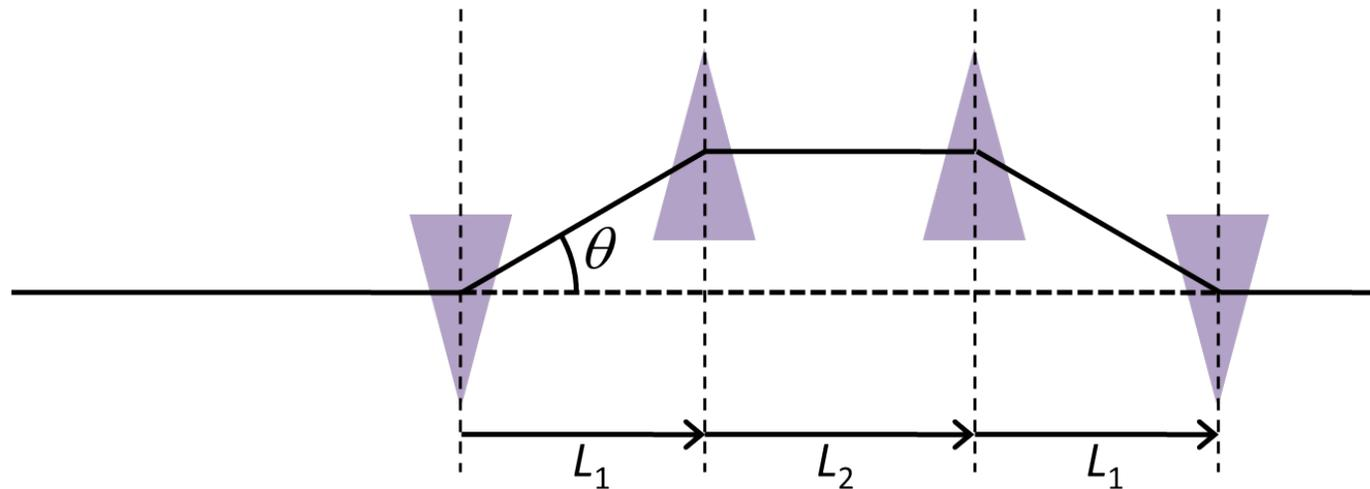
If we assume that the bending angle in a dipole is small,  $\theta \ll 1$ :
