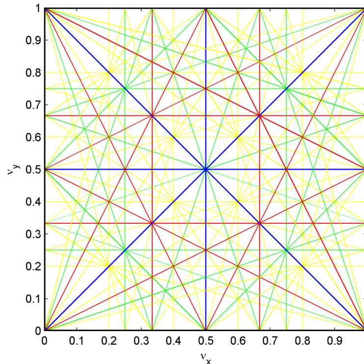
Resonances are associated with unstable motion for particles in storage rings.
