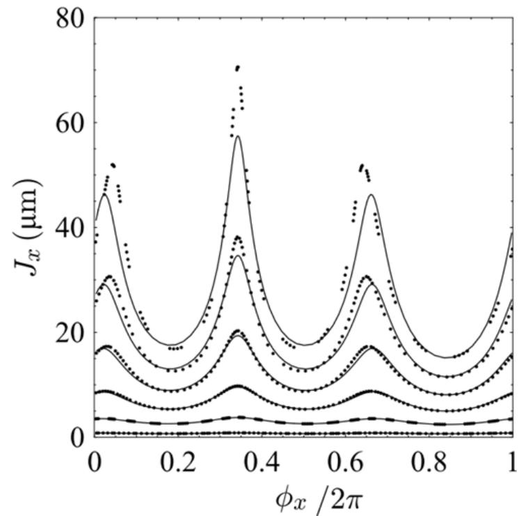
Close inspection of the plots on the previous slides reveals another effect, in addition to the obvious distortion of the phase space ellipses: the phase advance per turn (i.e. the tune) varies with increasing betatron amplitude.
