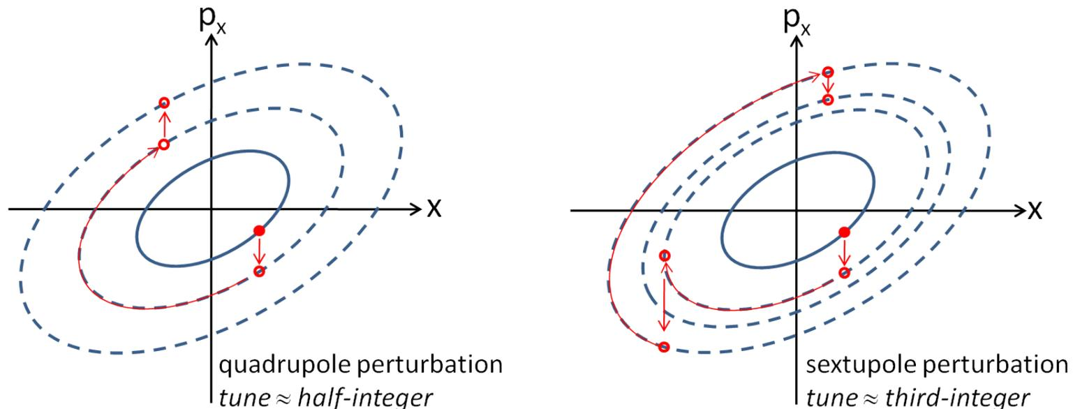
Higher-order multipoles drive higher-order resonances... but the effects are less easily illustrated on a phase space diagram.
