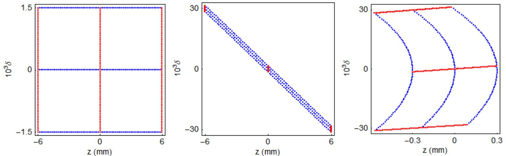
Although the bunch length has been reduced, there is significant distortion of the distribution: the rms bunch length will be significantly longer than we are aiming for.
