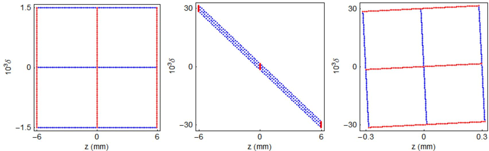
The rms bunch length is reduced by a factor of 20 as required, but the rms energy spread is *increased* by the same factor. This is because the transfer map is *symplectic*, so phase space areas are conserved under the transformation.
