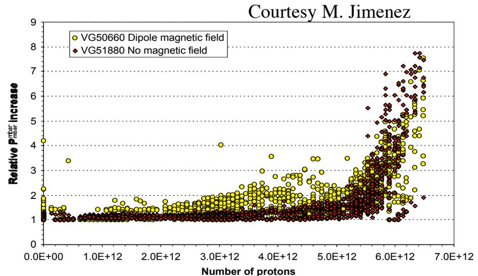
LHC cooling limit:  $P_{cloud} \sim 1 \text{ W/m} \rightarrow 10^{-6} \text{ mbar l/s/m}$
