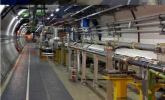
Beampipes in the long straight sections
