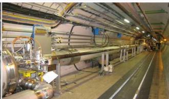
Beam dump line on top of circulating beams
