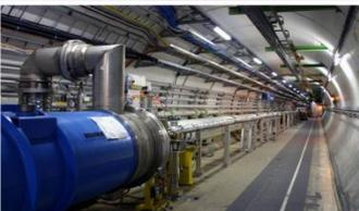
Beampipes in the long straight sections
