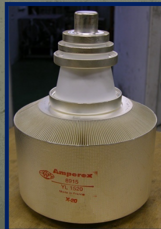
YL1520 (ex Philips, now Richardson), < 260 MHz, 25 kW
