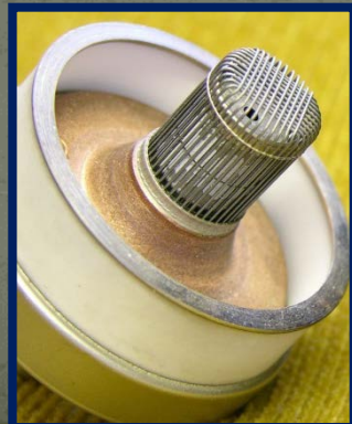
4CX250B (Eimac/CPI), < 500 MHz, 600 W (Anode removed)
