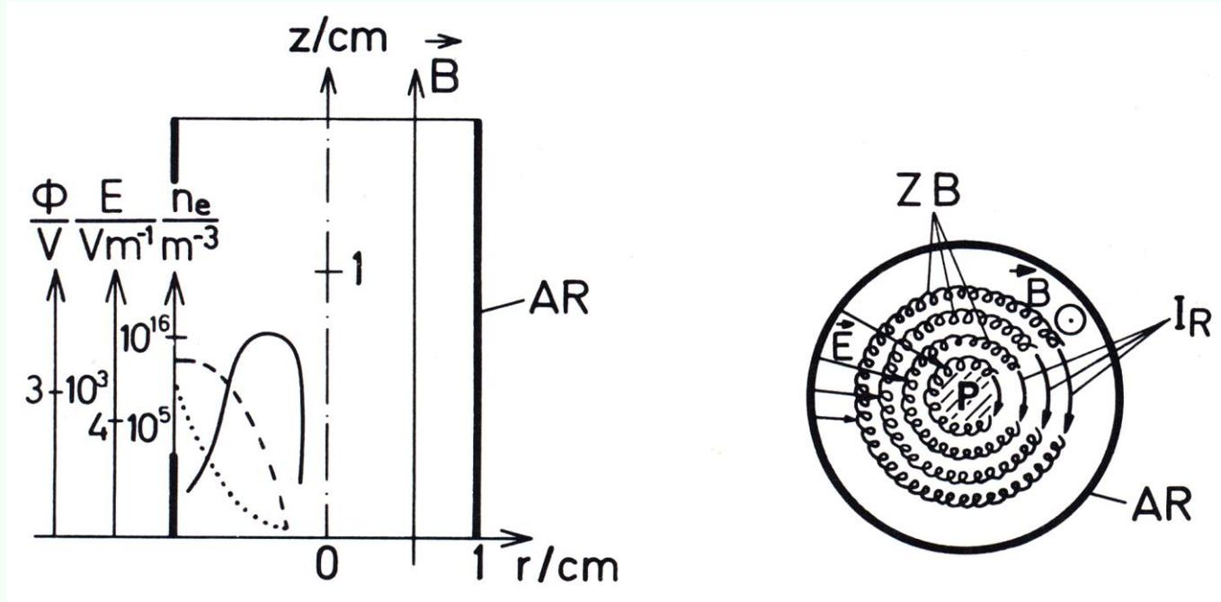
Field strength, potential, electron densities (left) and electron trajectories (right) in typical Penning gauge
