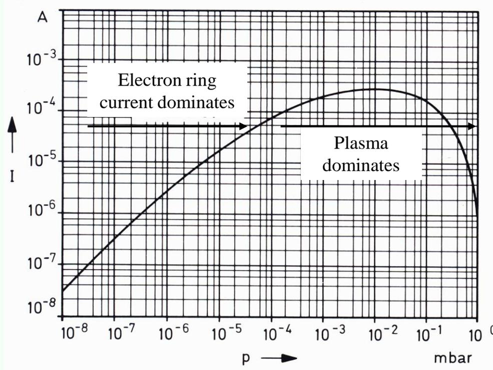
Calibration curve of typical Penning gauge
