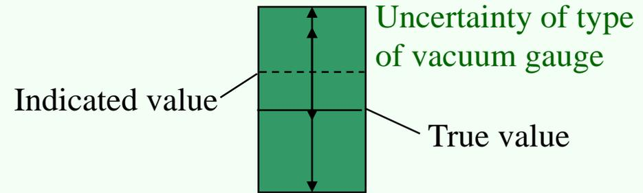
**Measurement uncertainty of a specific gauge:** Error of reading is known from calibration certificate and can be corrected!
