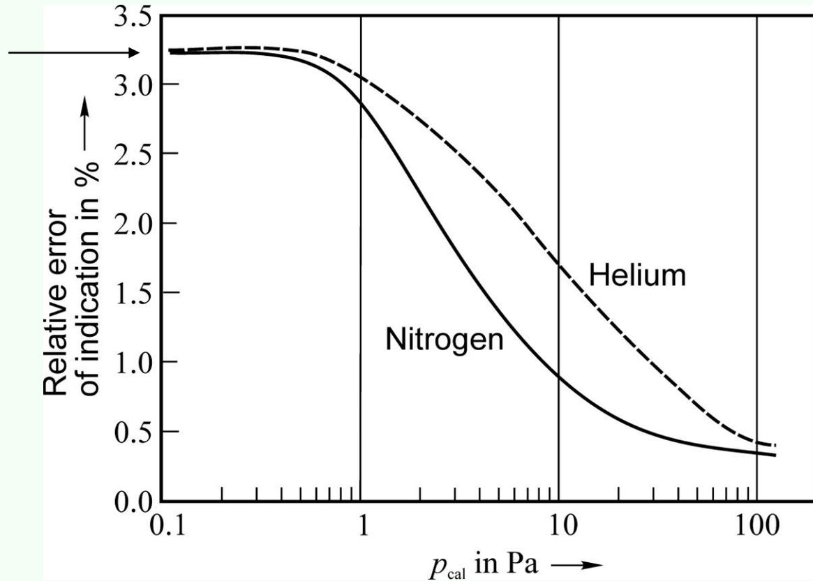
Calibration curve by PTB for two gases
