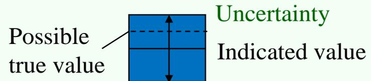
**Measurement uncertainty of a type of gauge:** Must include error of reading and uncertainty!
