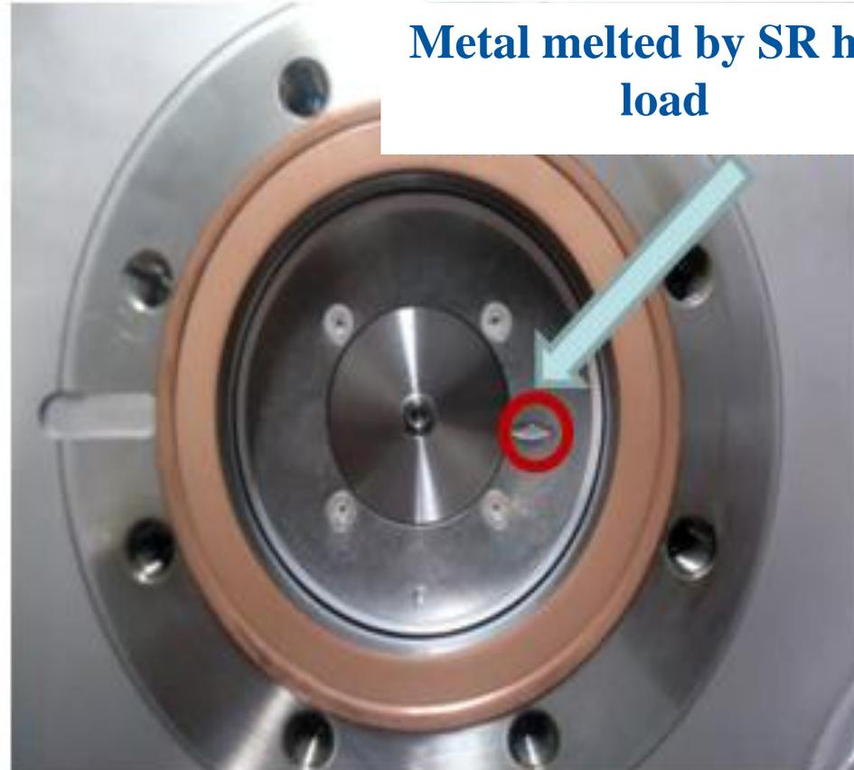
**Metal melted by SR heat load**
