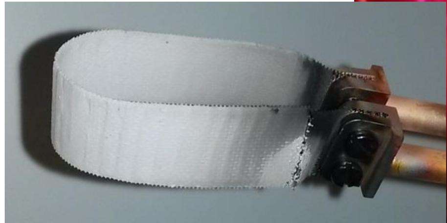
Failed cathode of the CERN duoplasmatron
