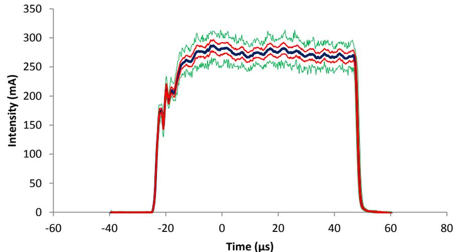
The plot shows the beam intensity out of the CERN Linac2 proton source. It includes H2+ and H3+, but H+ is ~200mA.
