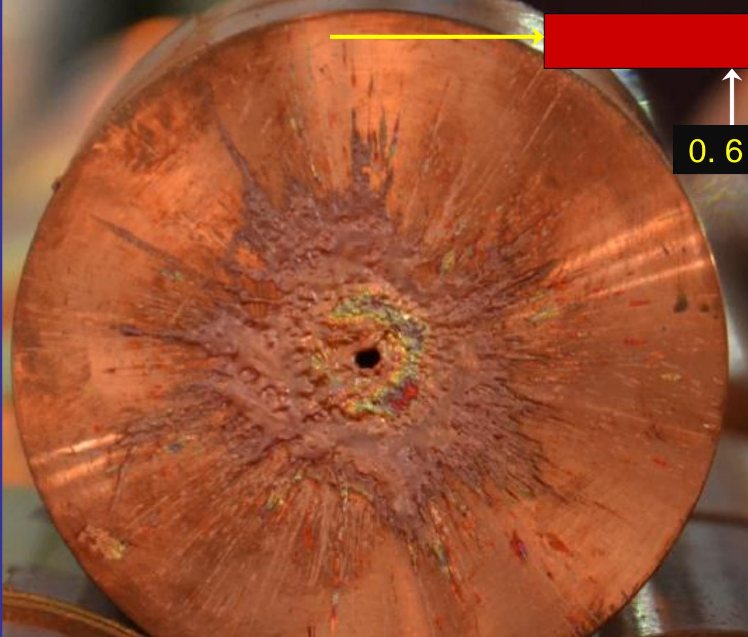
Copper part of a target at a depth of 0.6 m, irradiated with one SPS beam pulse (1.5 MJ, 7  $\mu$ s, 450 GeV, 0.2 mm)
