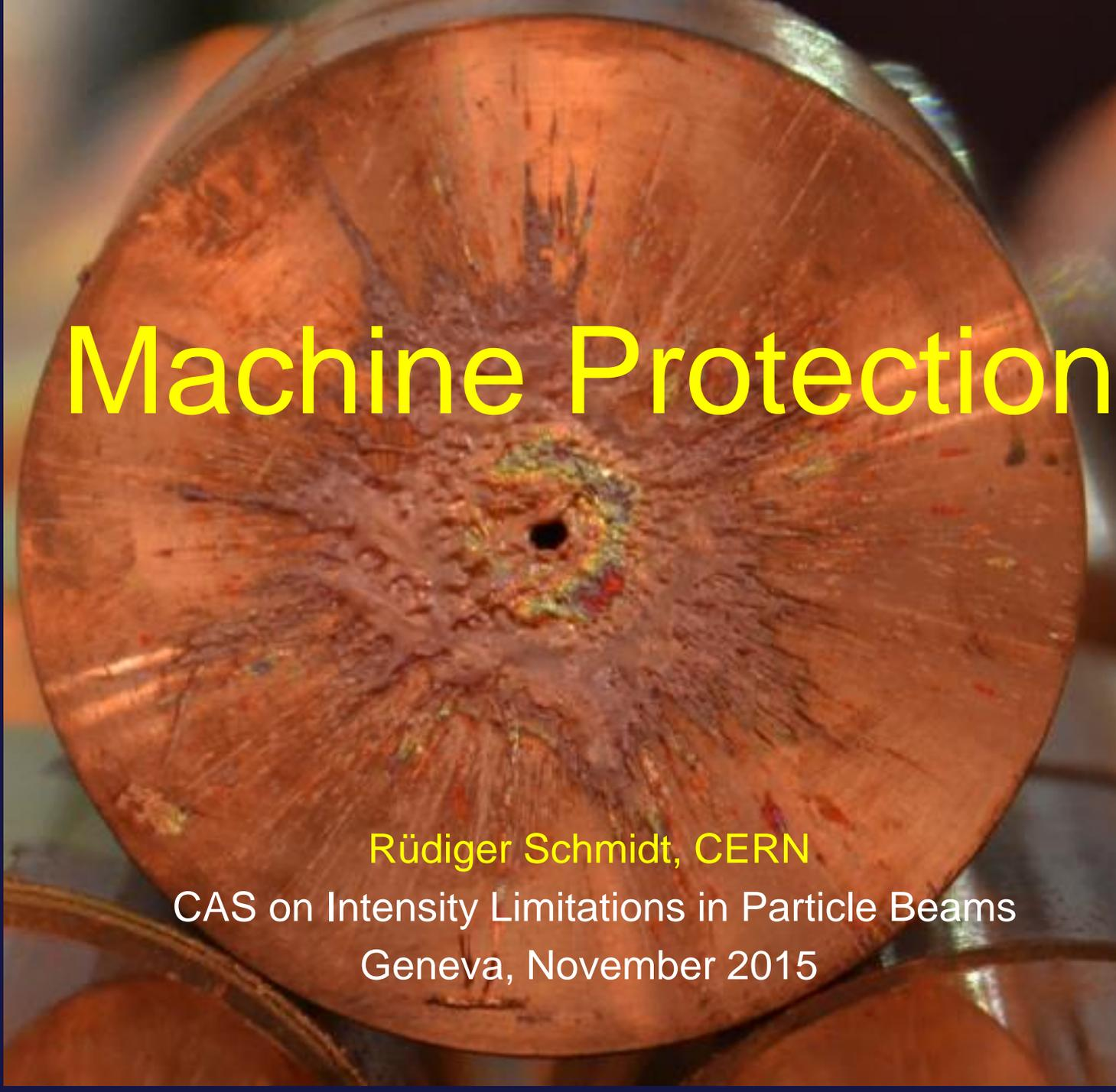
A close-up photograph of a circular copper beam pipe end. The surface is heavily scratched and shows a central impact point with a small hole and a colorful, crater-like residue, indicating significant damage from a particle beam.
