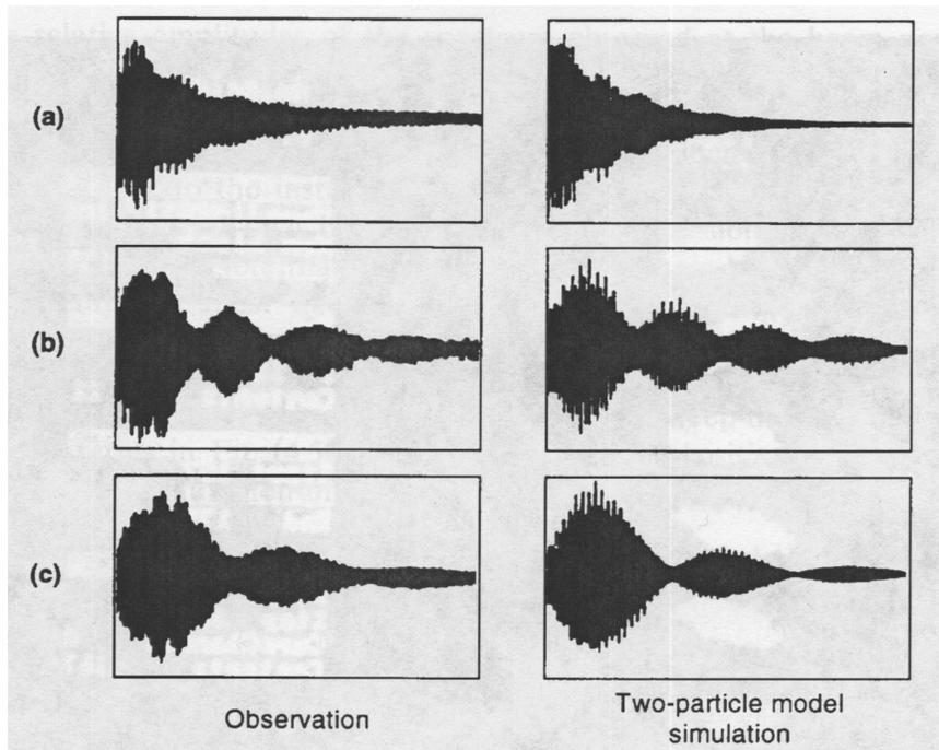
The beam-position-monitor signal as a function of time after the beam is kicked. Left: PEP data with (a)  $N/N_{\text{th}} = 0.86$ , (b)  $N/N_{\text{th}} = 0.93$ , and (c)  $N/N_{\text{th}} = 0.988$ . Right: two-particle model with (a)  $\Upsilon/2 = 0.77$ , (b)  $\Upsilon/2 = 0.96$ , and (c)  $\Upsilon/2 = 0.99$ .
