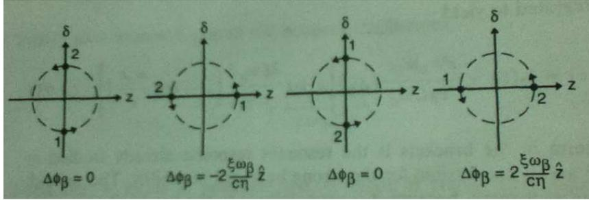
The synchrotron oscillations of a two-particle beam observed in the longitudinal phase space. The quantity  $\Delta\phi_\beta = \phi_{\beta 1} - \phi_{\beta 2}$  is the difference of the betatron phases of the two particles; it is modulated by the synchrotron motion as shown. The sense of rotation of particle motion in the phase space is for the case above transition, i.e.  $\eta > 0$ .
