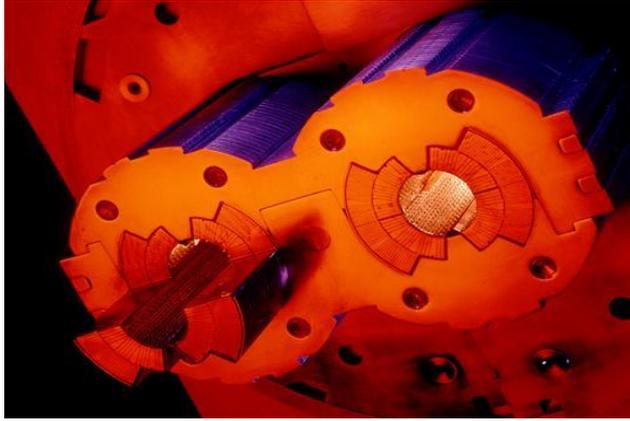
**Circular Orbit:** dipole magnets to define the geometry
