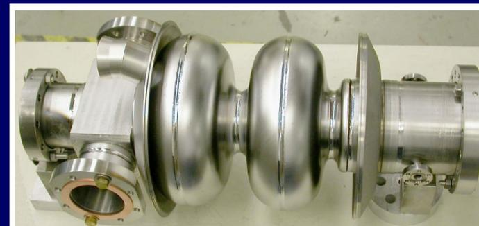
1.3 GHz, 2-cell cavity for Cornell ERL injector.
