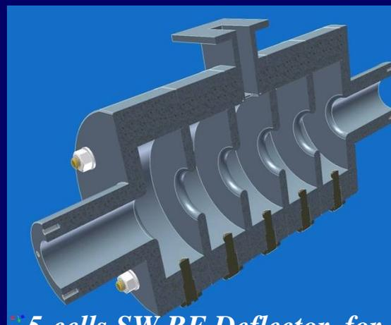
*5-cells SW RF Deflector for beam diagnostics at SPARC*
