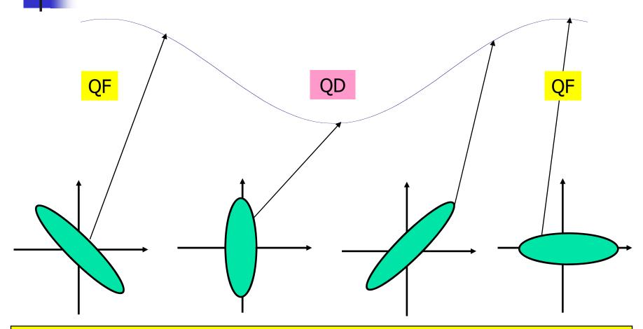
The shape of the ellipse varies along the machine, but its area (the emittance  $\varepsilon$ ) remains constant for a given energy.
