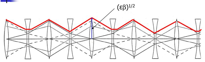
The  $\beta$ -function is the envelope around all the trajectories of the particles circulating in the machine.
