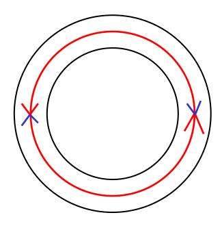
Colliders with the same type of particles (e.g. p-p) require two separate chambers. The beam are brought into a common chamber around the interaction regions
