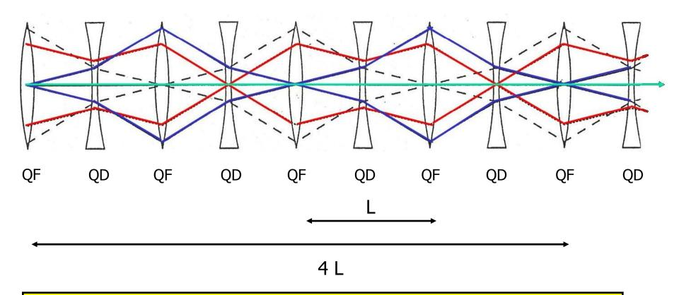
One complete oscillation in 4 cells  $\Rightarrow$  90°/ cell  $\Rightarrow \mu =$  90°
