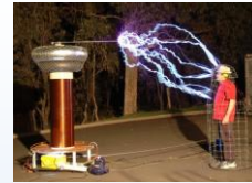
Faraday cage used to protect a person while demonstrating discharges from Tesla transformer
