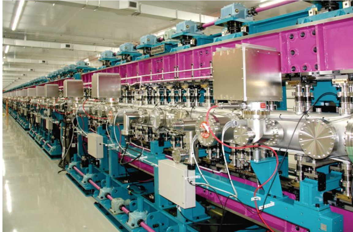
SACLA in-vacuum undulators (Japan XFEL)
