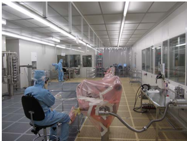
leak testing of a XFEL string
