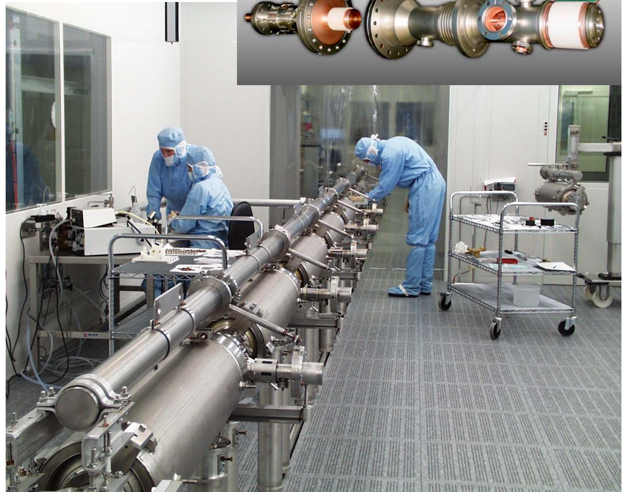
String assembly of 8 cavities for an XFEL module
