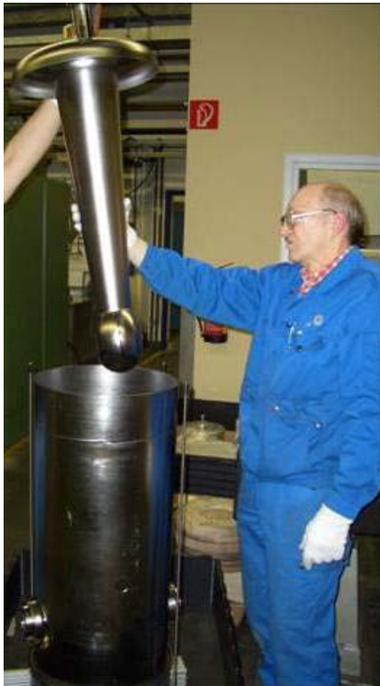
Assembly of the centre conductor of a quarter wave resonator
