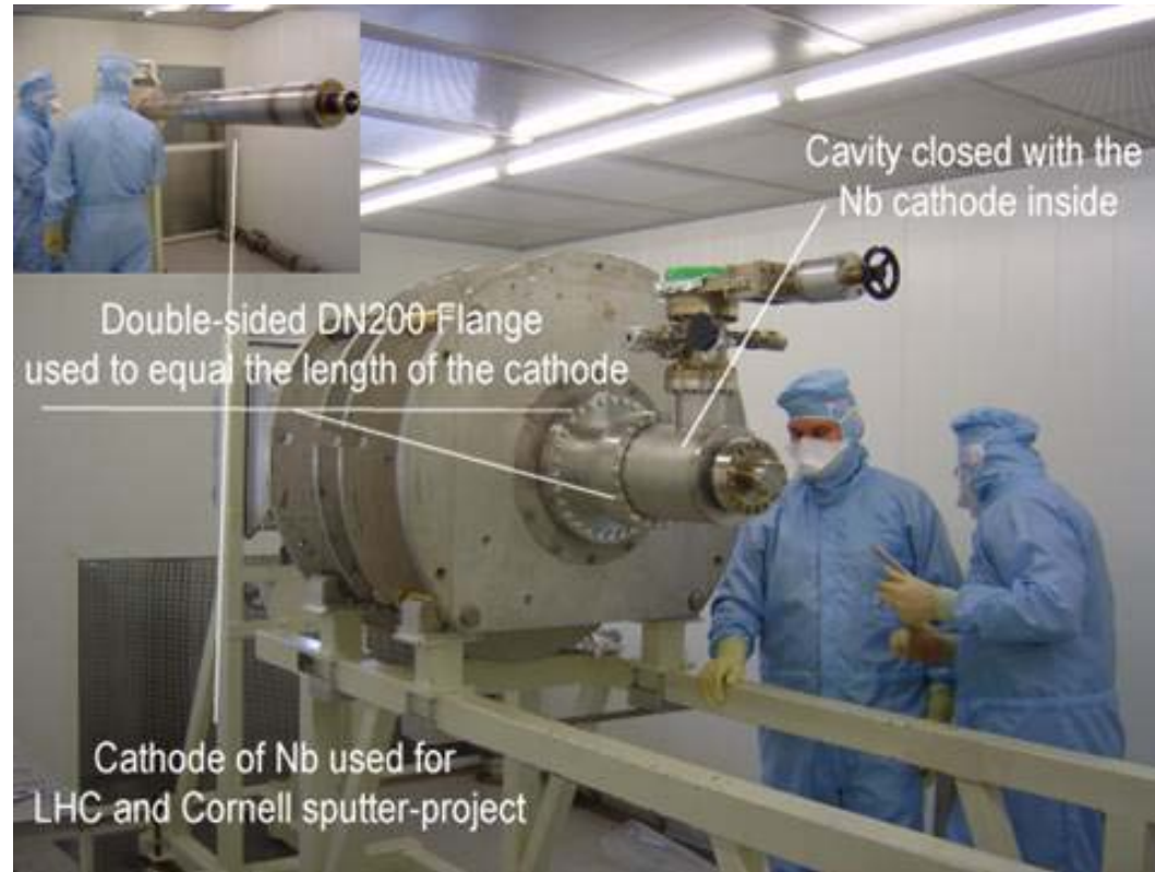
Assembly of the Niobium Cathode into a Copper cavity on the cavity axis
