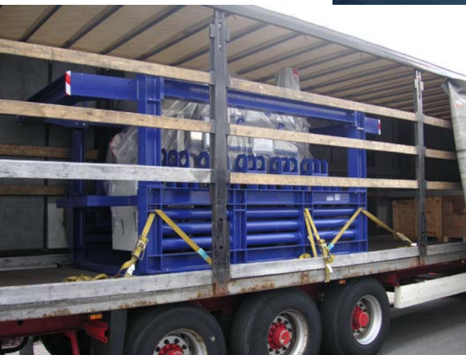
Land transport by truck with the srf module mounted to a special shock absorbing transport frame
