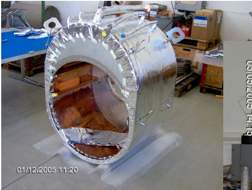
Heat Shield with cryogenic piping (LN2 cooling) and superinsulation foil
