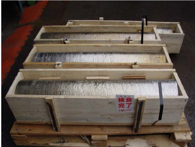
Nb ingot after refining by multiple electron beam welding in vacuum*
