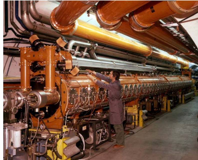
SPS Traveling Wave Cavity in the SPS tunnel. Backward Wave Structure, 90 degrees phase advance/cell, 200.22 MHz centre freq
