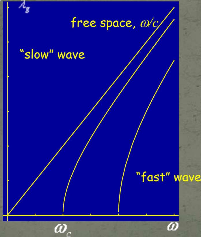
e.g.: TE<sub>10</sub>-wave in rectangular waveguide:
