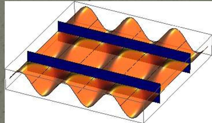
Metallic walls may be inserted where  $E_y \equiv 0$  without perturbing the fields. Note the standing wave in  $x$ -direction!
