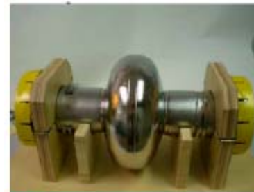
DESY single crystal cavity 1AC8 build from Heraeus disc by rolling at RWTH, deep drawing and EB welding at ACCEL
