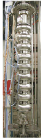
60mm-Aperture Re-Entrant Cavity, 58 MV/m! KEK/Cornell Collaboration
