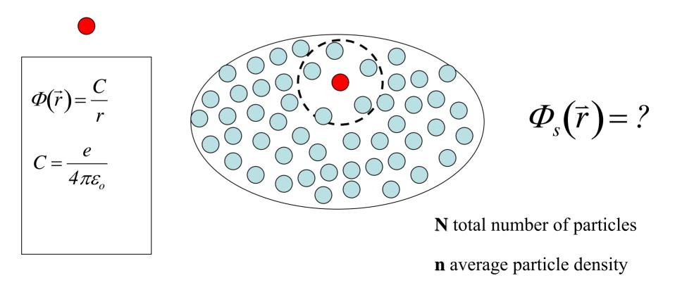
The effective potential of a test charge can be defined as the sum of the potential of the uniform distribution and a "perturbed" term.
