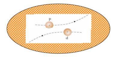
2) **Space Charge Regime** ==> dominated by the **self field** produced by the particle distribution, which varies appreciably only over large distances compare to the average separation of the particles ==> **Collective Effects**
