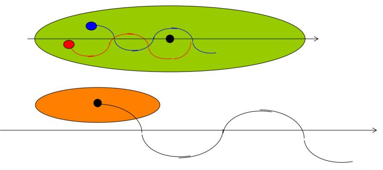
These force may have a complicate dependence on the charge position. A simple analysis is done considering only the linear expansion of the self-fields forces around the equilibrium trajectory.
