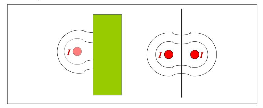
In analogy with the image method for charges close to conducting screens, we get the magnetic field, in the region outside the material, as superposition of the fields due to two symmetric equal currents flowing in the same direction.
