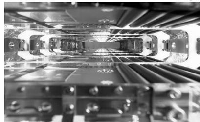
electrodes installed inside magnets
