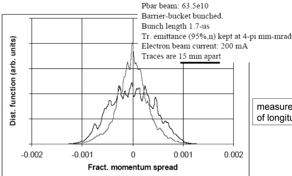
measured by detection of longitudinal Schottky noise
