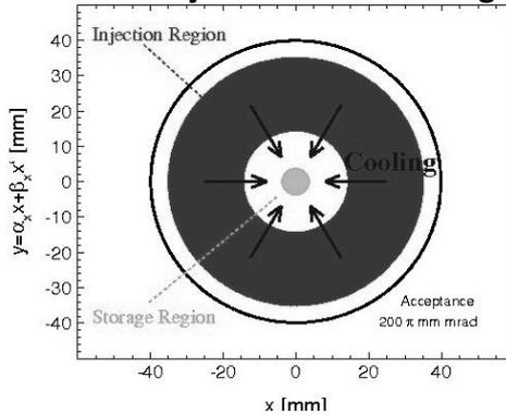
fast electron cooling of highly charged ions ( $\text{Au}^{63+}$ ) at injection energy allows accumulation with a repetition rate of 5 Hz
