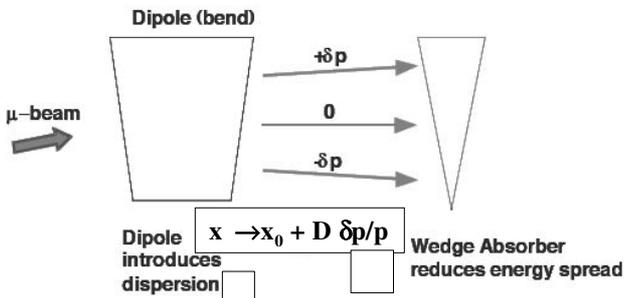
$$\frac{d\sigma_E^2}{ds} = -2 \frac{\partial(dE/ds)}{\partial E} \sigma_E^2 + \frac{d\langle \Delta E_{rms}^2 \rangle}{ds}$$
