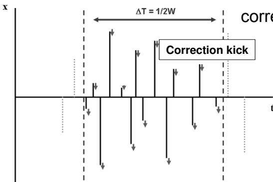
correction kick  $\Delta x = \frac{g}{N_s} \times \sum_{i=1..N_s} x_i$ ,  $N_s = N \frac{\Delta T}{T_0} = \frac{N}{2WT_0}$
