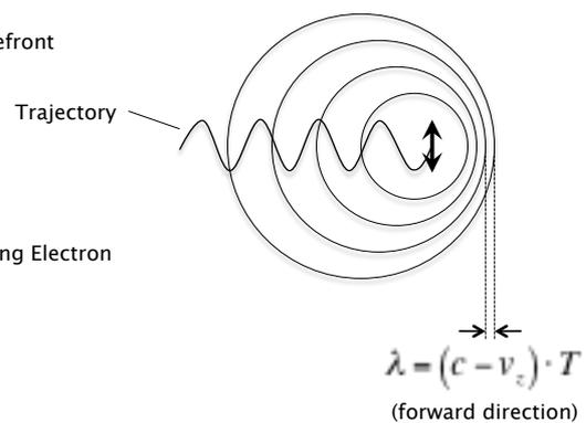
For relativistic electrons the longitudinal velocity  $v_z$  is close to  $c$ , resulting in very short wavelength (blue shift of photon energy)
