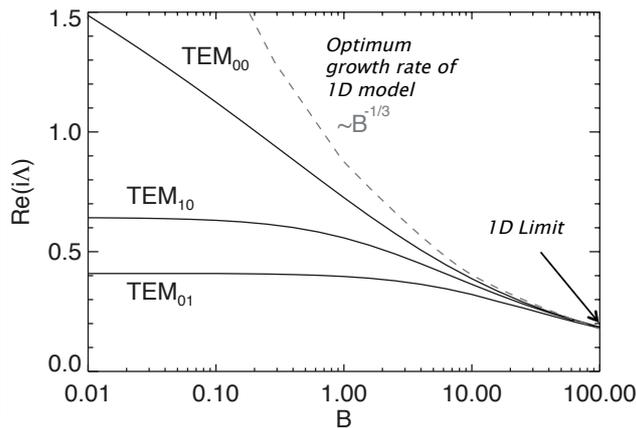
← Increased gain length due to strong diffraction
