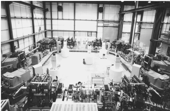
Example: heavy ion storage ring TSR 8 dipole magnets of equal bending strength
