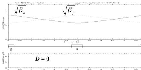
optical functions of a FoDo cell without
