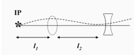
$$\beta(s) = \left(1 + \frac{l_2}{f_1}\right)^2 * \beta^* + \frac{1}{\beta^*} \left(l_1 + l_2 + \frac{l_1 l_2}{f_1}\right)^2$$
