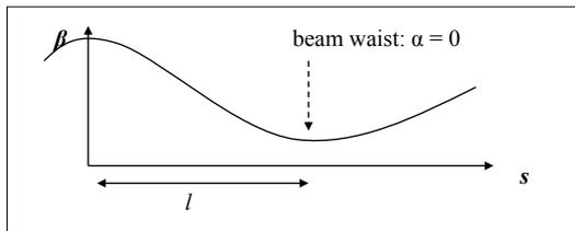
given the initial conditions  $\alpha_0, \beta_0, \gamma_0$ : where is the point of smallest beam dimension in the drift ... or at which location occurs the beam waist ?
