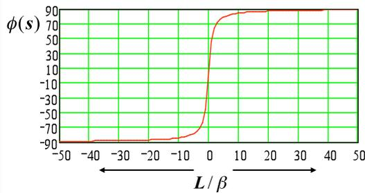
Consider the drift spaces on both sides of the IP: the phase advance of a mini  $\beta$  insertion is approximately  $\pi$ , in other words: the tune will increase by half an integer.
