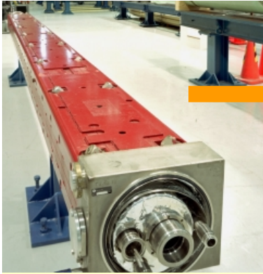
Tevatron dipoles: 4.2 T single aperture, warm yoke
