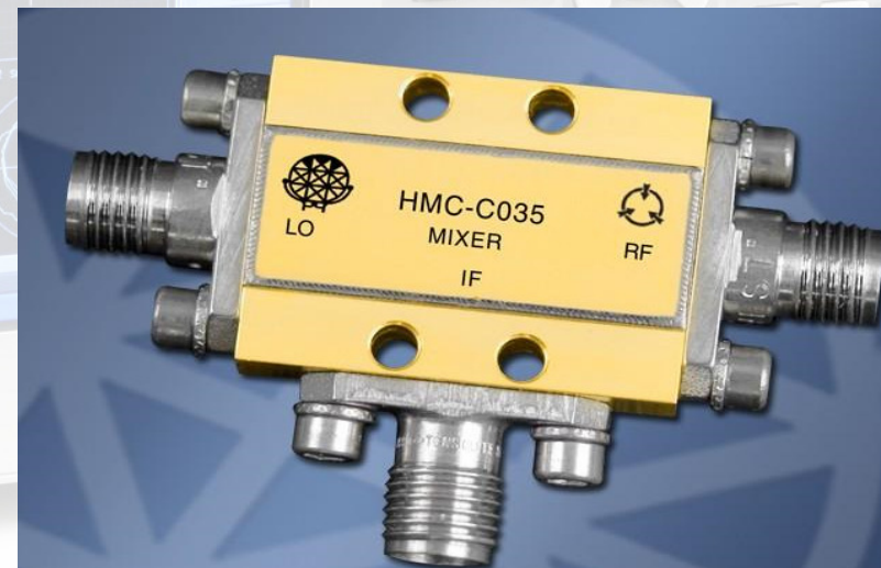
◆ A typical coaxial mixer (SMA connector)
