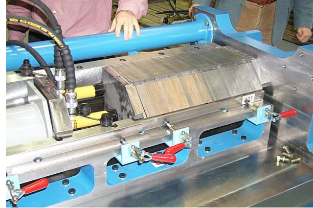
Double aperture LHC quad. MQW Stacking on a precision table
