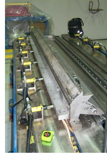
Double aperture LHC quad. MQW Stacking on a precision table
