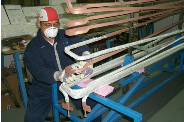
MQW Glass fibre tape wrapping.
