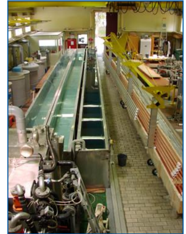
cuves for beam screens
