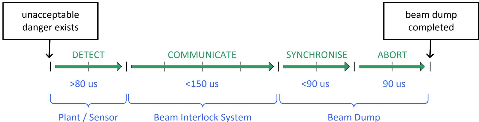
At the LHC the delay can be up to  $\sim 3$  turns –  $\sim 300 \mu\text{s}$ .
