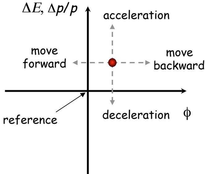
The particle trajectory in the phase space ( $\Delta p/p, \phi$ ) describes its longitudinal motion.
