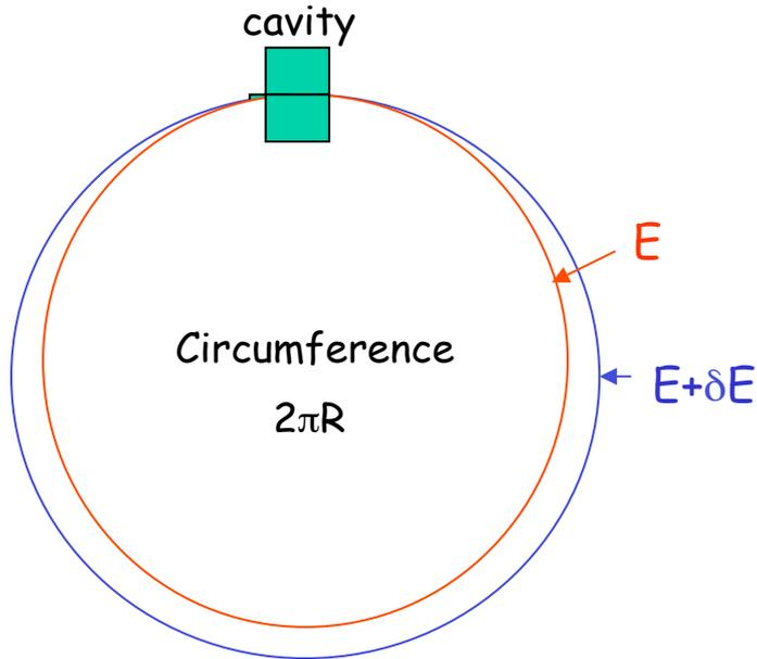
If a particle is slightly shifted in momentum it will have a different orbit and the orbit length is different.
