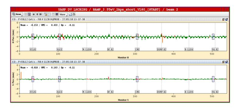
A measured closed orbit in LHC, 540 beam position monitors
