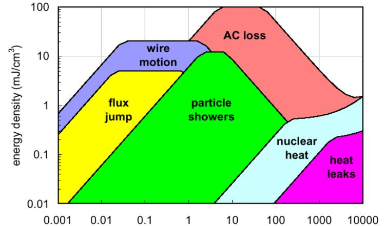
With stored energies > MJ the coils can overheat if nothing is done ( $T = 3000\text{K}$  is possible ! )
