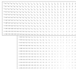
The e.m. forces in a quadrupole magnet tend to push the coil
