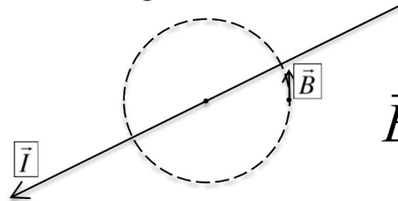
If you wanted to make a  $B = 8$  T magnet with just two infinitely thin wires placed at 50 mm distance one needs :  $I = 5 \cdot 10^5$  A
