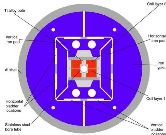
Fig. 2. HD2 cross-section.
