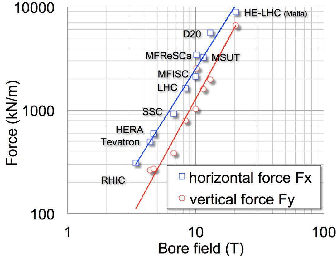
The electromagnetic loads in a 20 T dipole would be a factor 5 to 8 larger than in the LHC dipoles
