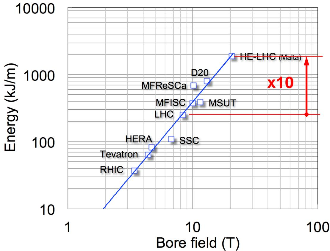
Scaling of the energy per unit length of magnet in recent production vs. R&D dipoles
