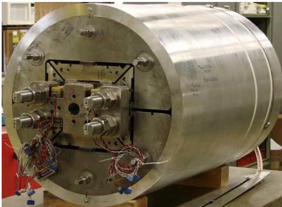
Fig. 1. HD2 assembled and pre-loaded.
