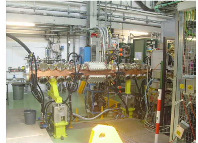
The CERN Linac4 RFQ 45 keV – 3 MeV, 3 m 80 mA H-, max. 10% duty cycle
