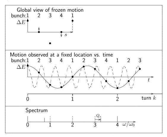
M equidistant bunches have M independent modes of coupled bunch oscillations labeled  $0 \le n \le M-1$  related to oscillation phase difference  $\Delta \phi$  of adjacent bunches  $n = \Delta \phi/(2\pi M)$ . Each mode n has one pair of sidebands in each frequency range of  $M\omega_0$
