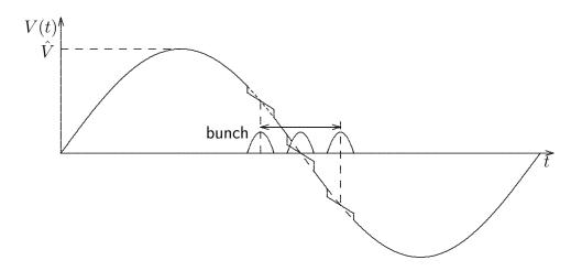
Only the incoherent frequency of individual particles changed (reduced for  $\gamma > \gamma_T$ , increased for  $\gamma < \gamma_T$ ). The coherent dipole (rigid bunch) is not affected. This separates the coherent synchrotron frequency from the incoherent distribution and leads to a loss of Landau damping. The reduction of longitudinal focusing increases the bunch length given by a 4th order equation for protons with constant phase space area
