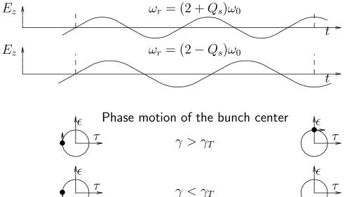
The growth rate is given by the side-band impedance difference
