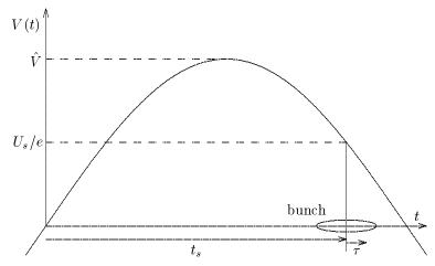
With an RF cavity of voltage  $\hat{V}$  and frequency  $\omega_{\rm RF}=h\omega_0$  and a SR energy loss per turn U the energy gain or loss  $\delta E$  is
