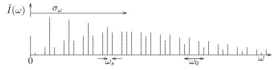
A bunch executes a synchrotron oscillation with frequency  $\omega_s = \omega_0 Q_s$  and amplitude  $\hat{\tau}$ . It gives a modulation of its passage time  $t_k$  at a cavity in successive turn k
