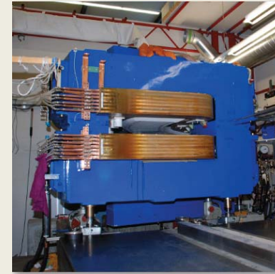
40 Tons-90° AMF3 dipole 1.5 T, G=0.15m
