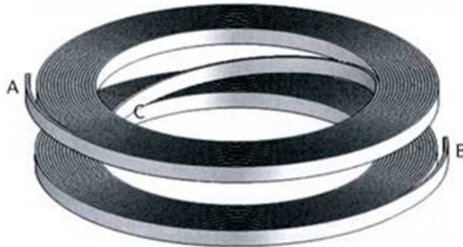
Fig. 3.23 Pictorial view of a double-pancake coil, with the top and bottom pancakes separated axially for clarity. The pancakes in this drawing are wound with a tape conductor. Points A and B indicate the ends of a continuous conductor, with Point C marking the approximate midpoint.
