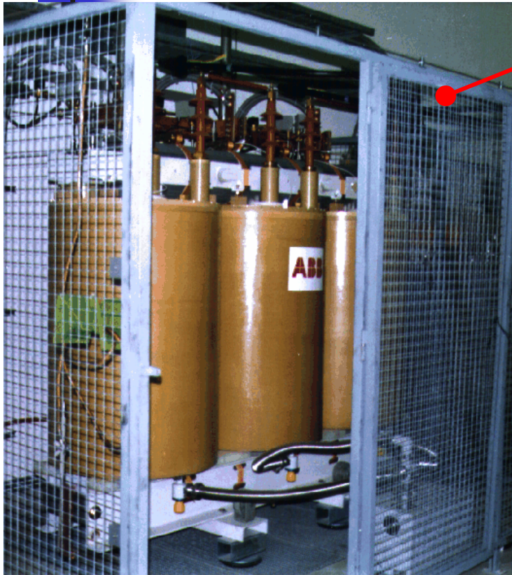
Toroidal magnet of 200 kJ / 160 kW energy store ( B = 4 \text{ T} , dia. = 1.1 m)
