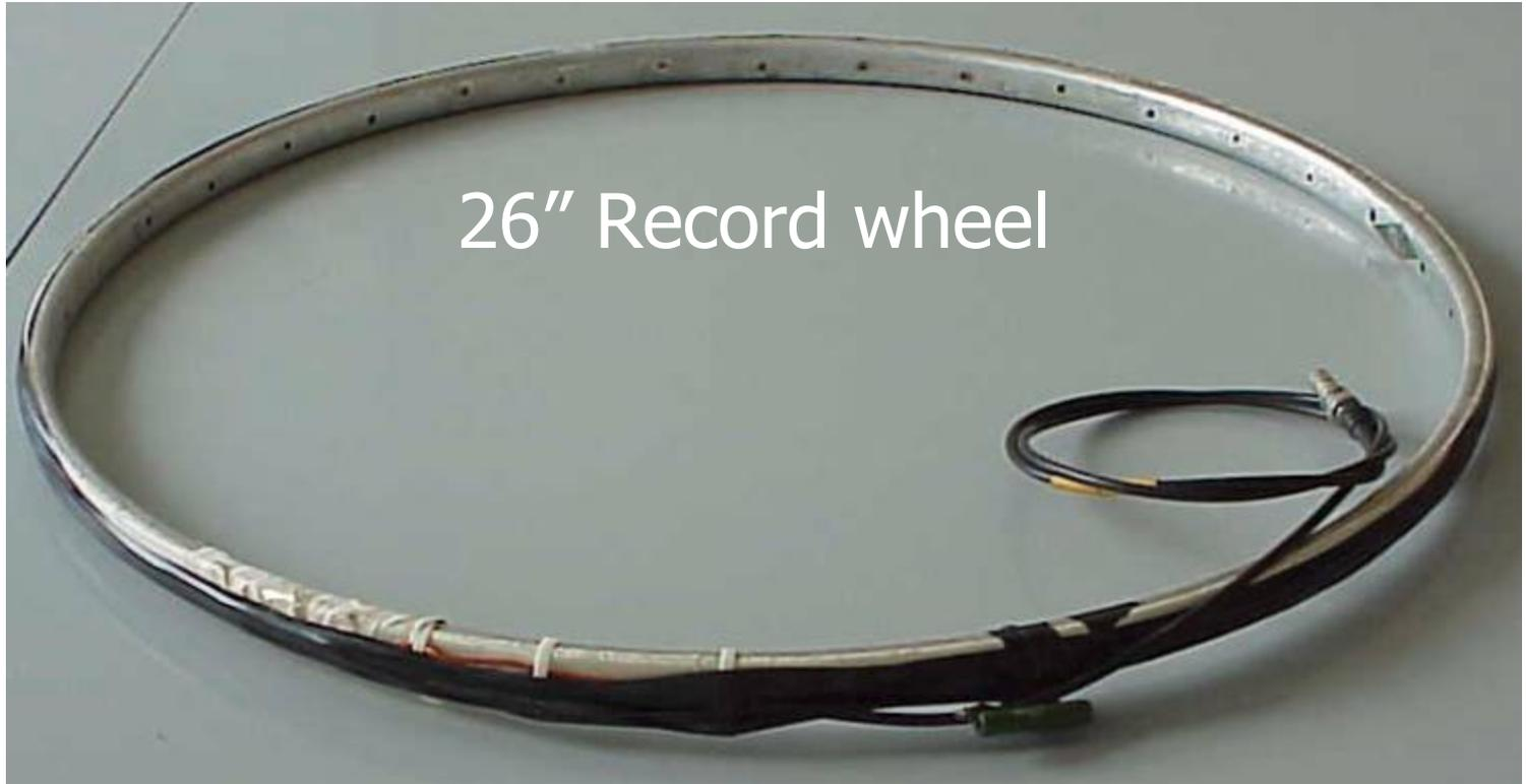
... no, actually this is a *fixed coil* with 800 turns and  $\approx 250 \text{ m}^2$  surface that has been used to verify e.m. coupling of LEP and SPS
