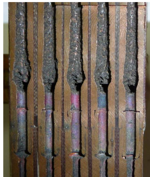
Cooling Water speed too high. Excessive cavitation and erosion
