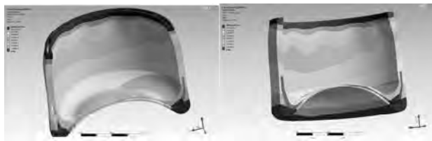
Stresses in the beam entrance window due to off center beam
