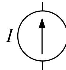
Similar to the voltage sources this can be extended to elements which current can not have discontinuities.
