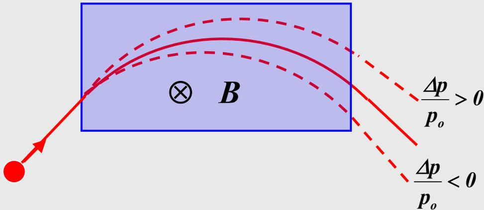
Particles with different energies are moving on different orbits in a bending magnet →
