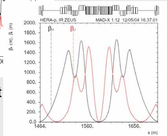
HEP colliders are composed by long regular FODO cells in the arcs and a few low beta insertions:
