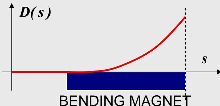
A rectangular magnet corresponds to a drift in the horizontal plane and the optical functions  $\alpha$ ,  $\beta$ ,  $\gamma$  inside have a simple relations to the initial values at the entrance of the magnet:
