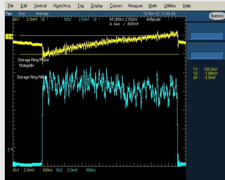
Phase variation along the bunch train (for a partially filled ring) causes a split in frequency for the individual bunches and therefore a suppression of longitudinal multi-bunch instabilities
