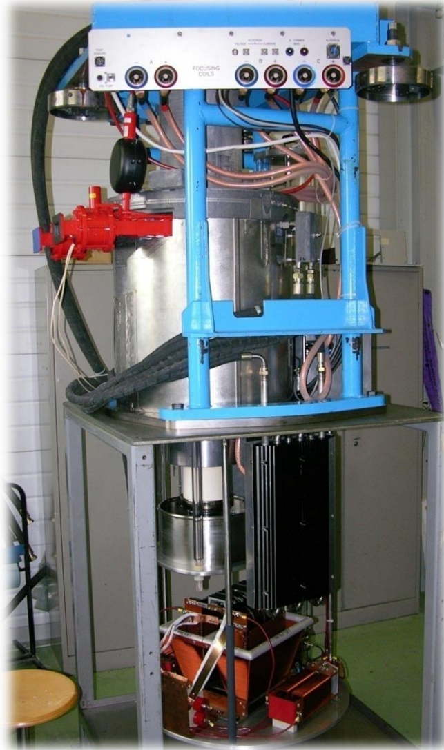
CERN CTF3 (LIL): 3 GHz, 45 MW, 4.5 \mu s, 50 Hz, \eta 45 %
