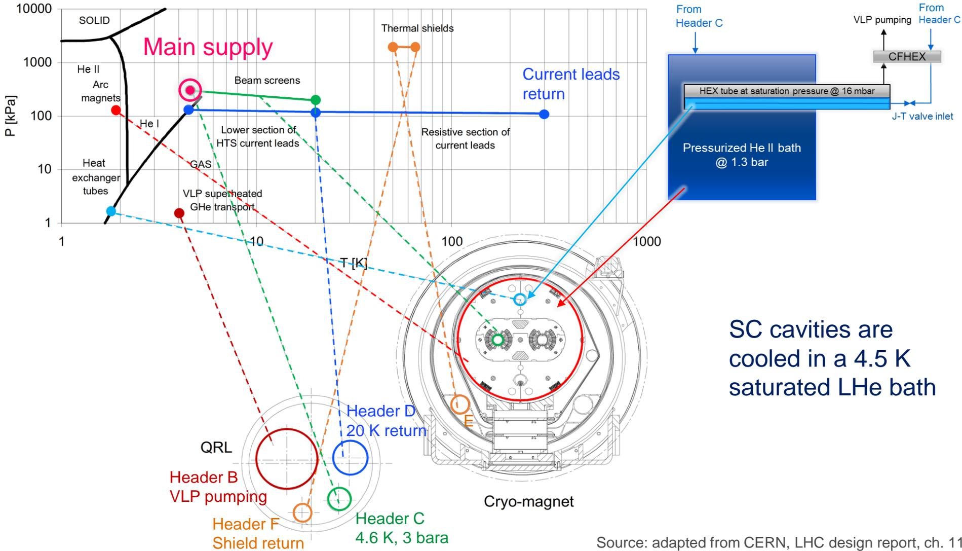
SC cavities are cooled in a 4.5 K saturated LHe bath
