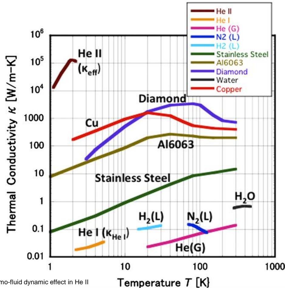
Murakami, Experimental study of thermo-fluid dynamic effect in He II cavitating flow, Cryogenics, 2012.
