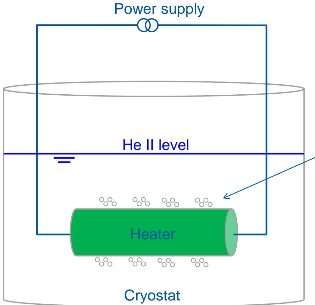
Heat and mass flow are limited by a critical velocity:
